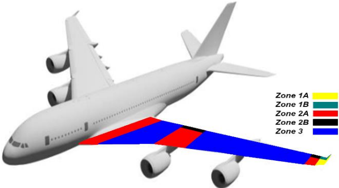
Figure 2.1: Lightning strike zones of an aircraft wing.
